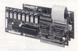
All Bufferboard features are controlled by its own unique on-board micro controller, including the Bufferboard's automatic memory configuration. This feature eliminates the need to change switch setting when additional chips are installed. Also, the Bufferboard is equipped with its own built-in RAM Diagnostic Self Test, which alerts the user of any abnormal conditions related to the memory chips.
