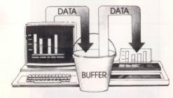
Thanks to the Bufferboard, your system is now operating at its maximum speed and efficiency. You can continue your data processing while your printer finishes the previous job.
